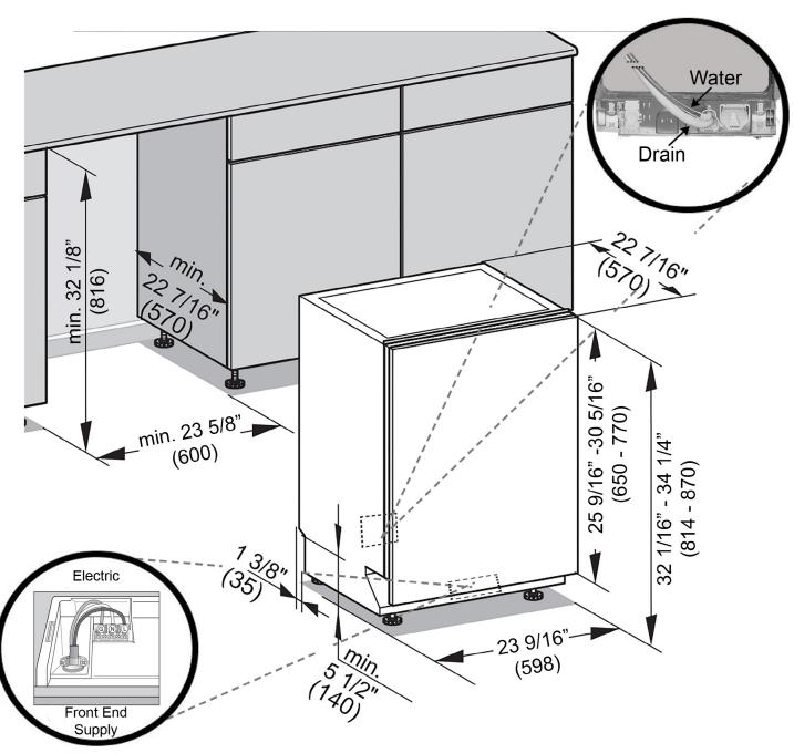
**Drain** - 4 ft 11 in (1.5 m) flexible drain hose. (Connects from lower center rear)
